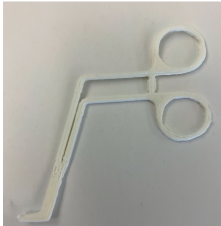
Figure 2: 3-D printed device from the CAD file shown in Figure 1
